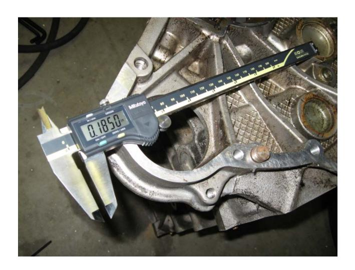
Proceed to cut the first socket cap screw down to a few thou less than the value on the previous page using a hacksaw or one of those thin disc-cutters in you angle grinder
