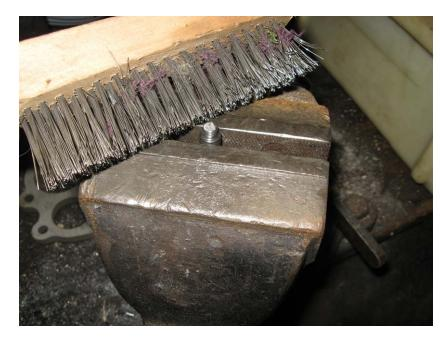
Wind the screw into the hole, being careful not to cross-thread it. If it doesn't start easily, then put it back on the vise and file a little more around the lead of the thread. Torque it up snug. In the image below, you can see I am checking if the screw is proud using my fingers. It is easy to feel for this. In this case, the front face of the screw is proud of the liner. This will foul the piston skirt, so it needs more taking off.
