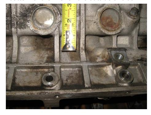
The area shown inside the red in this image shows the ideal location to drill holes for the pinning operation. This area ends up approx ¾" below the lower oil control ring so there is no concern with any interfering with the rings.
