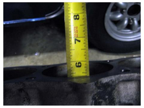
The bottom of the measure shows the bottom of the liner on the outside of block
