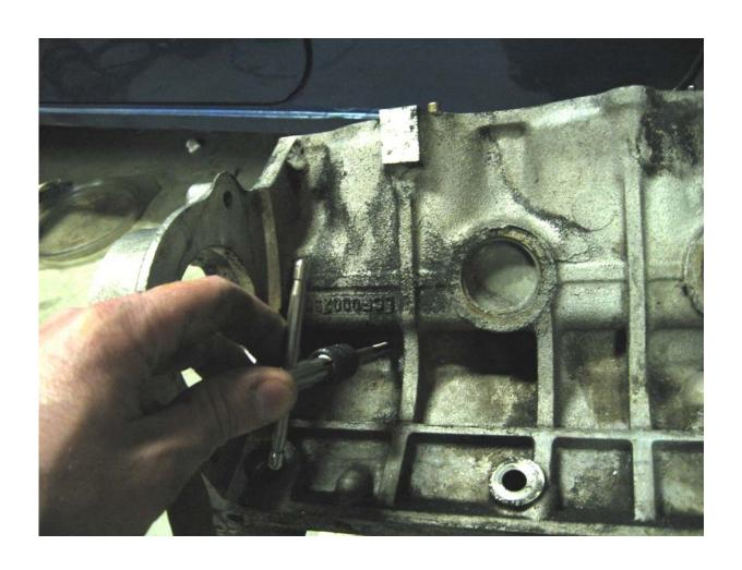
Now that the drilling and tapping is complete, reach inside the liner, and with a small piece of emery cloth, or wet/dry paper, gently rub around the hole. This will remove any small burrs left that could scuff the piston.
