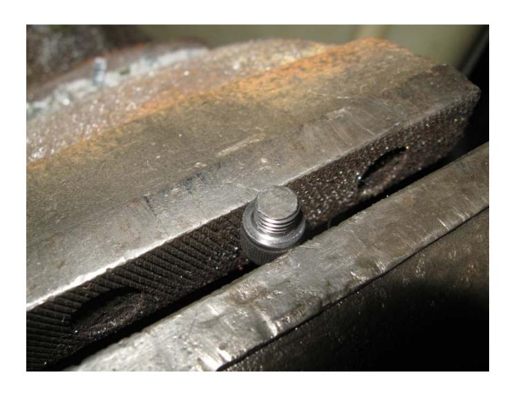
The tip of the screw is now sitting just inside of the liner – the feel test with your finger is enough to verify this. Now, it is time to remove the screw, and clean down the thread and area with brake cleaner one last time. After this is done, put some loctite on the screw thread, and wind it back in. It doesn't need to be really tight, just snug. The last thing you want to do is strip the thread.
