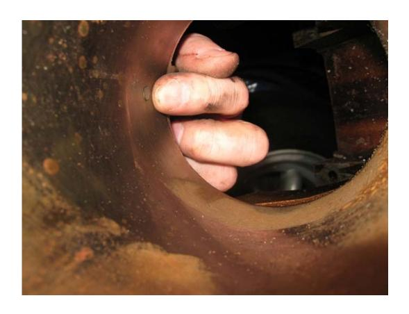
The screw has now been filed down some more to make it shorter and the lead-thread chamfered slightly to make it start easily in the threaded hole.
